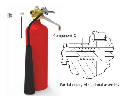
(a) Component C was modelled using 3D CAD.
