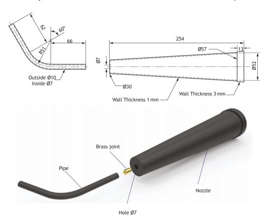
(b) Describe the 3D CAD modelling techniques used to create the **pipe** component. Refer to the dimensions given in the drawing.
