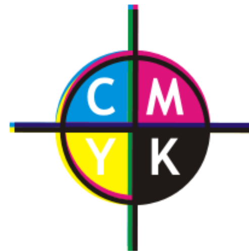
Exaggerated example of a mismatch of CMYK registration
